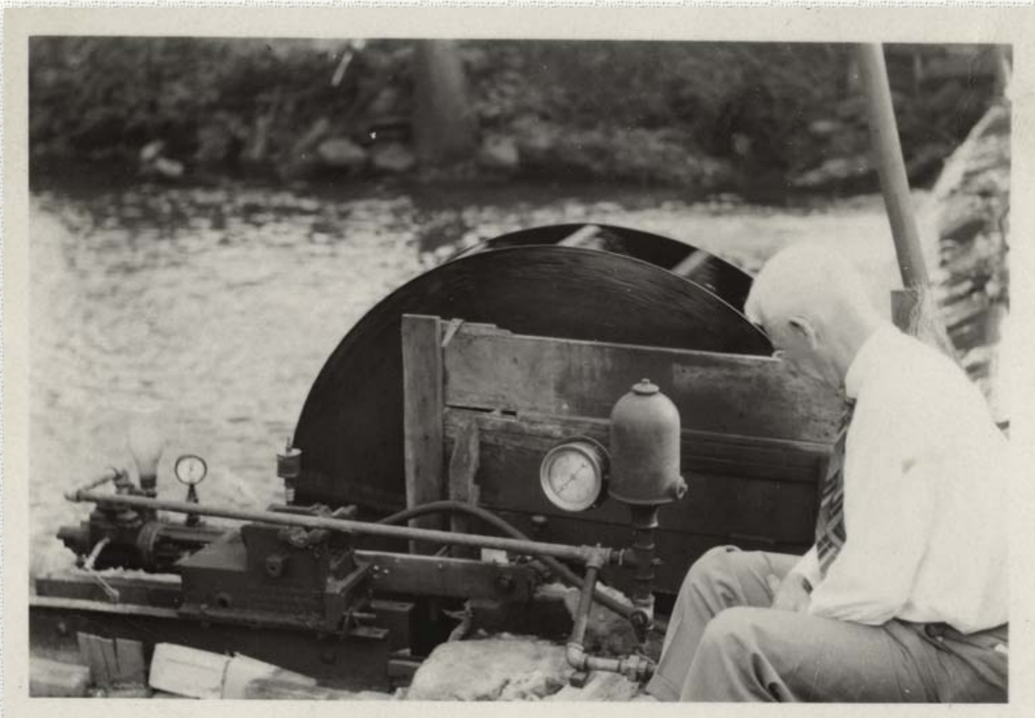
LeRoy Beers – a happy man at play. The water wheel drove an electric generator and mechanically pumped water to an above-ground tank on the hill above the garden. The gravity-fed system was used for irrigation and two decorative fountains. One was in the garden and one in a goldfish pond on the lower level.
